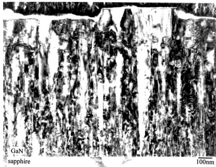
Figure 1. TEM image illustrating the high density and diverse range of dislocations, domain boundaries, basal plane stacking faults and surface facets that can form within MBE grown GaN/sapphire.
